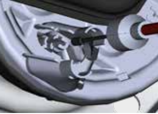
Hook-in Bowden cable saves assembly time.
