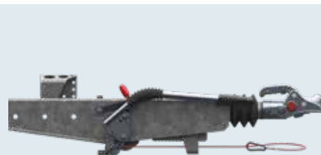
Handbrake lever opened = brake rod not clamped
