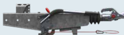
Handbrake lever applied = brake rod clamped, handbrake lever lowered
