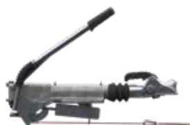
Handbrake lever closed (parking brake forwards)
