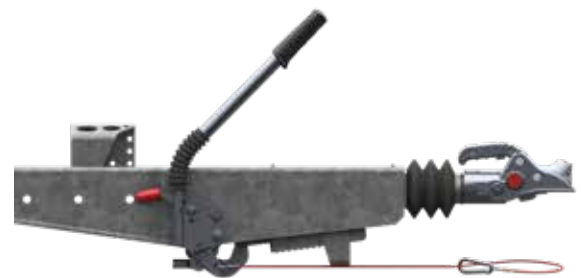
Handbrake lever closed (parking brake forwards)
