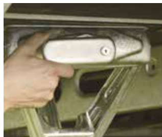
Insert the security device into the slot and push to the right
