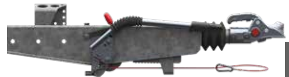
Handbrake lever opened (driving)
