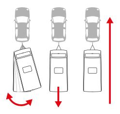
The driving behaviour of the caravan is permanently controlled by the ATC. Sensors detect dangerous lateral movements directly on the caravan axle, even before an ESP system for trailers installed in the car is able to sense the pendulum movement. The caravan will immediately — without any action on the part of the driver — brake gently and return to a stable driving condition.
