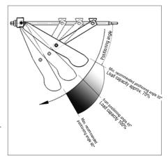
AL-KO corner steadies achieve their maximum load capacity from a positioning angle of 45° onwards. If the corner steady is positioned at a very flat angle (e.g. 30°), the load capacity will be reduced (see diagram).
