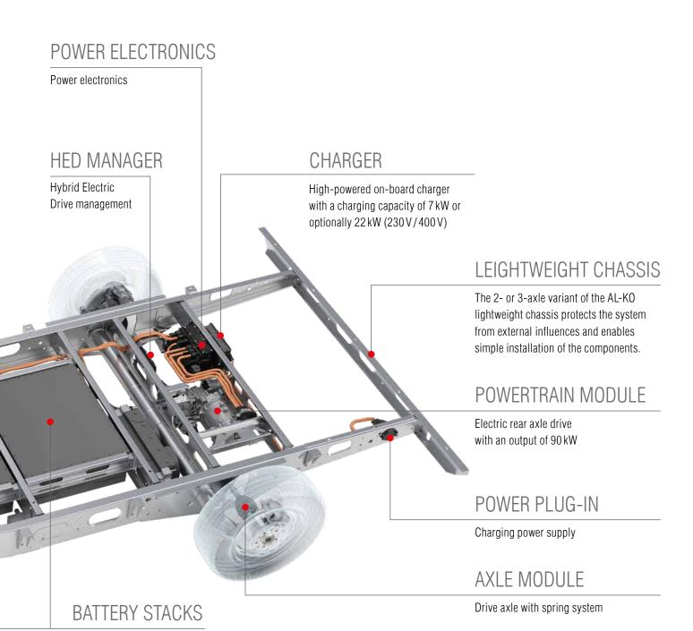
Scalable battery modules with a possible range of up to and over 100 km
