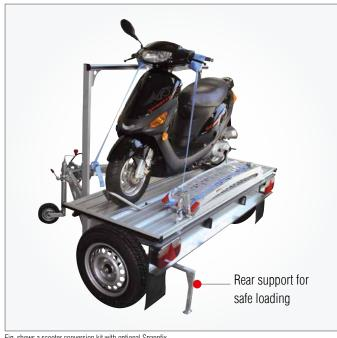
$\label{eq:Fig.Shows} \textbf{Fig. shows a scooter conversion kit with optional Spannfix}.$
