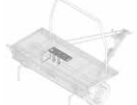
Spare wheel carrier for vehicle wheel
